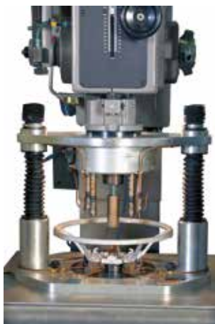
Detail of drilling with a multiple head for automobile steering wheels.
