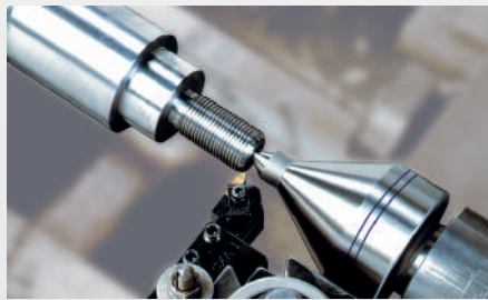
The extended running point guarantees the required clearance angle for turning parts with small diameters.
