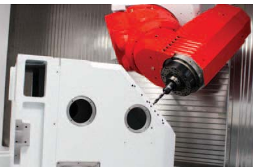
Milling, drilling and tapping on a milling head holder saddle
