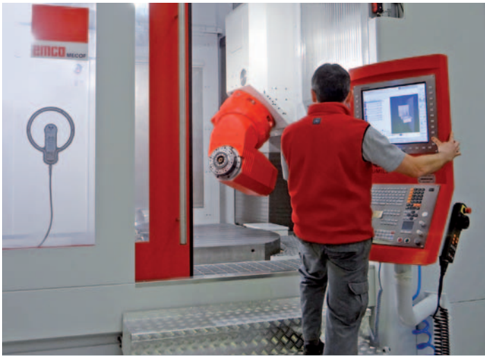
Ergonomic operation. Featuring two swivel joints, the operating panel can be pivoted into the work space.
