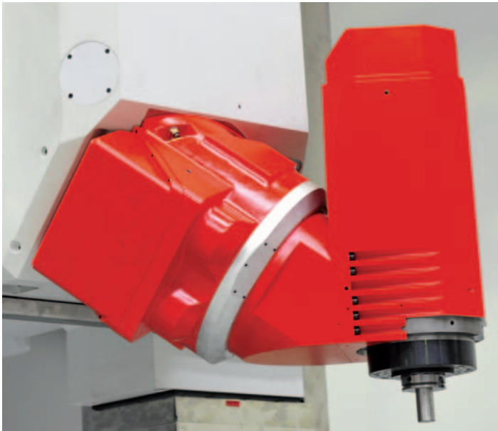
Electric spindle. Compact design with high-performance electric spindle. Continuously variable universal head offering high dynamics for simultaneous machining in connection with the NC rotary table.
