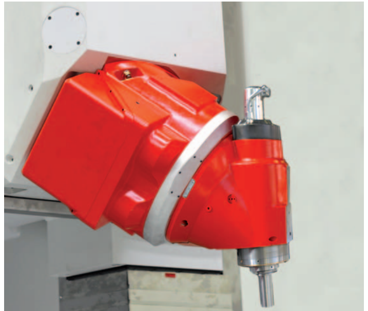
Mechanical spindle. Powerful mechanical spindle with high torque and high rigidity for heavy-duty and multi-sided machining in one setup.
