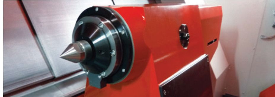
Tailstock with quill with CM5 or optionally with CM6 always with integrated bearing for stable process support.
