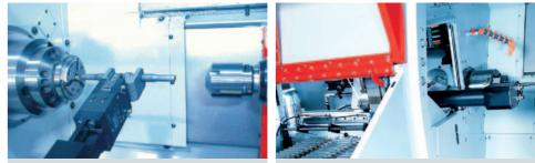
Multiple infeed chutes for loading rotationally symmetrical blanks. A sensor monitors the availability of blank parts for each infeed chute
