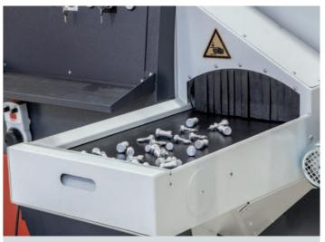
**Finished parts conveyor.** The parts catcher deposits the finished parts on an accumulating conveyor with a usable storage area of 340 x 750 mm.
