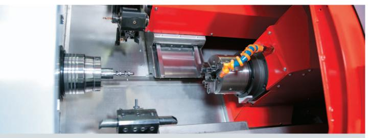
**Work area.** The generous work area provides space for several tools on both turrets and ensures a continuous chip flow even when few machine technicians are at work. Additional coolant pumps and a sophisticated pipe system clears the chips into the chip conveyor.
