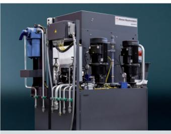
Band filter system with high-pressure coolant pumps A coolant pressure of 25/40/60/80 bar can be set as necessary. This enables coolant-fed drilling and milling tools to be used to their best advantage
