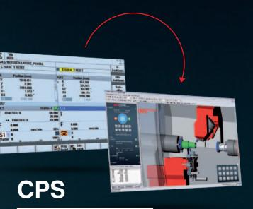
1:1 simulation with collision detection
