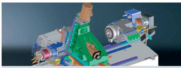
**Y-axis.** The Y axis is integrated into the basic machine structure and stands at 90° to the X axis. Extremely short projections form the basis for solid turning and drilling operations and also for milling operations without interference contours.
