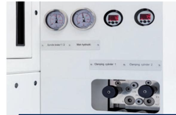
**VALVE BLOCK FOR ADJUSTING THE CLAMPING PRESSURE**
