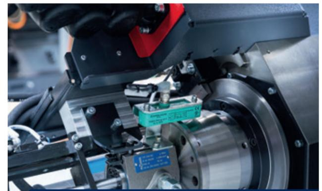
**CLAMPING STROKE CONTROL ON THE MAIN AND COUNTER SPINDLE**
