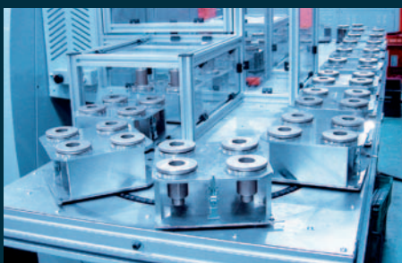
4-station pallet attachment for valve caps
