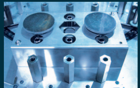
Multi-pallet attachment for a family of parts
