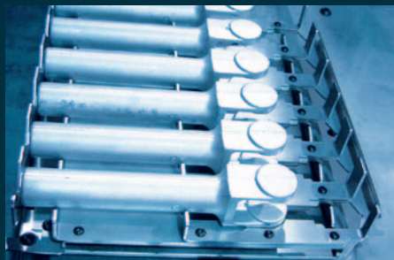
6-station pallet attachment for articulated brackets
