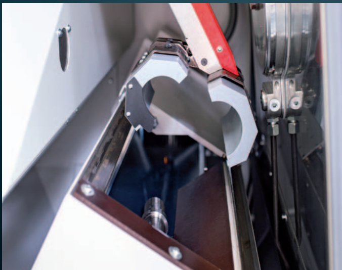
Parts catcher. The HYPERTURN 65's electro-pneumatic parts catcher is controlled using M functions. When needed, it traverses to the front of the work area and pivots to the spindle center. The finished part is removed from the clamping device and transferred to the catcher tray. The parts catcher then moves back to its initial position and the part is tipped onto a conveyor belt.
