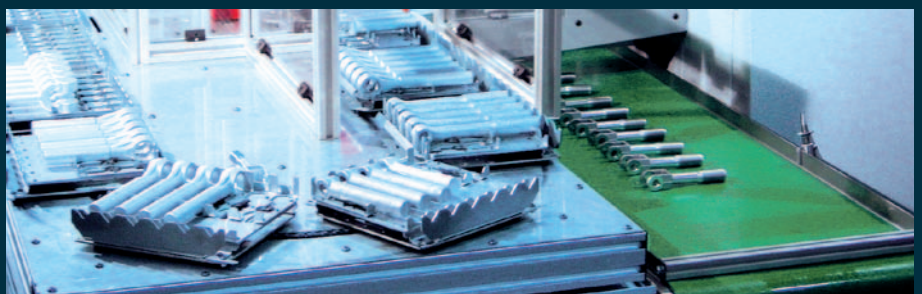
20-station pallet magazine with customer-specific pallets
